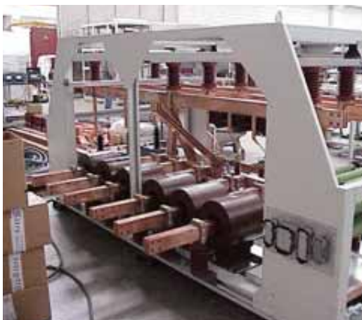
> AGN-24 Transformer for generator switchgear.
