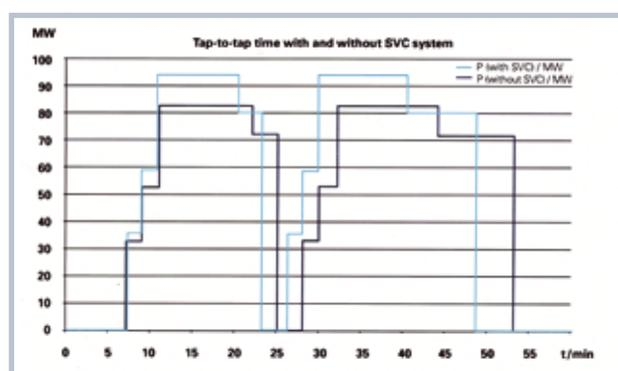
This figure shows the influence of the shortened tap-to-tap time as increased steel production. The melting time of the changes decreased from 53 minutes to 48 minutes once the SVC was installed. This is a 9.4% reduction of one heat time - the total increase of the productivity can be transferred to the steel tons via saved time for each heat.
