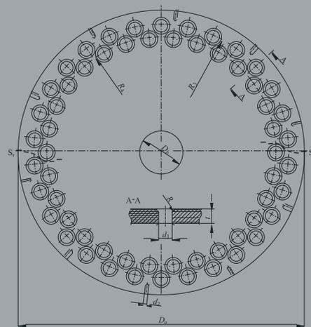
**Continuous disc windings** are made of several numbers of equal coils or sections connected in series. These windings are of advantage when used for transformers rated above 2500 kVA and rated voltages upto 145 kV.
