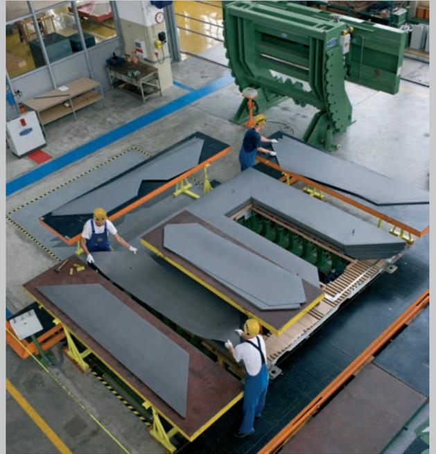
The core laminations are securely held together by means of heat shrinkable polyglass bands and tightening facilities made from anti-magnetic steel in such a way that movement of laminations during transportation and vibrations during operation are prevented.
